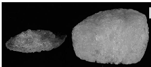
Figure 7 Side view of the polyester foams. Height comparisons between two citric acid : glycerol molar ratios, 0.5 : 1 (left) and 1.4 : 1 (right) given 60 s microwaving. Bar = 10 mm.
